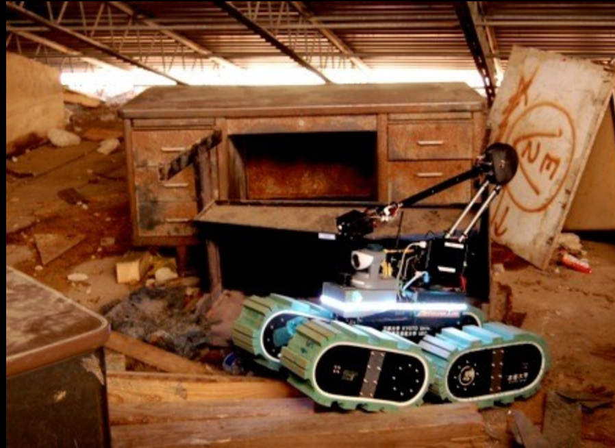
KOHGA3 ground robot (shown here during a test) to inspect a collapsed building in Hachinohe, in the northeastern portion of Honshu island
