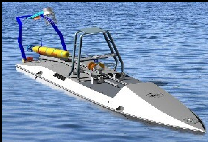
USV Equipped With UUV Handling System brooke-ocean.com
